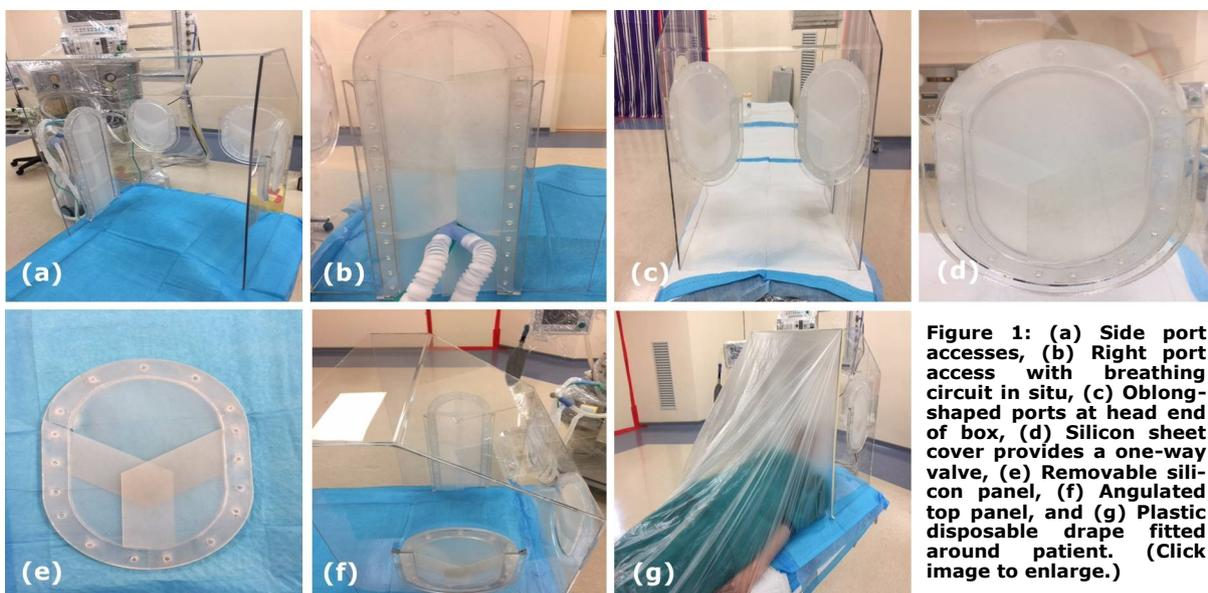
**Figure 1:** (a) Side port accesses, (b) Right port access with breathing circuit in situ, (c) Oblong-shaped ports at head end of box, (d) Silicon sheet cover provides a one-way valve, (e) Removable silicon panel, (f) Angulated top panel, and (g) Plastic disposable drape fitted around patient. (Click image to enlarge.)
